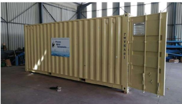
3m 3 /hr Containerised Reverse Osmosis Plant - Botswana
